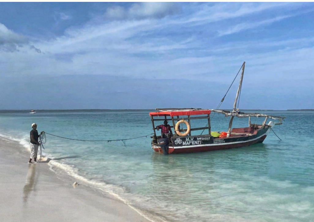
Dhow MAPENZE and Captain Zakarya of Kendwa, NW coast of Zanzibar, Tanzania. For tourists, Captain Z constructed an ugly 'room addition' frame fitted with a cheap plastic tarp to make her a "shade boat" to protect against the searing hot equatorial sun.
